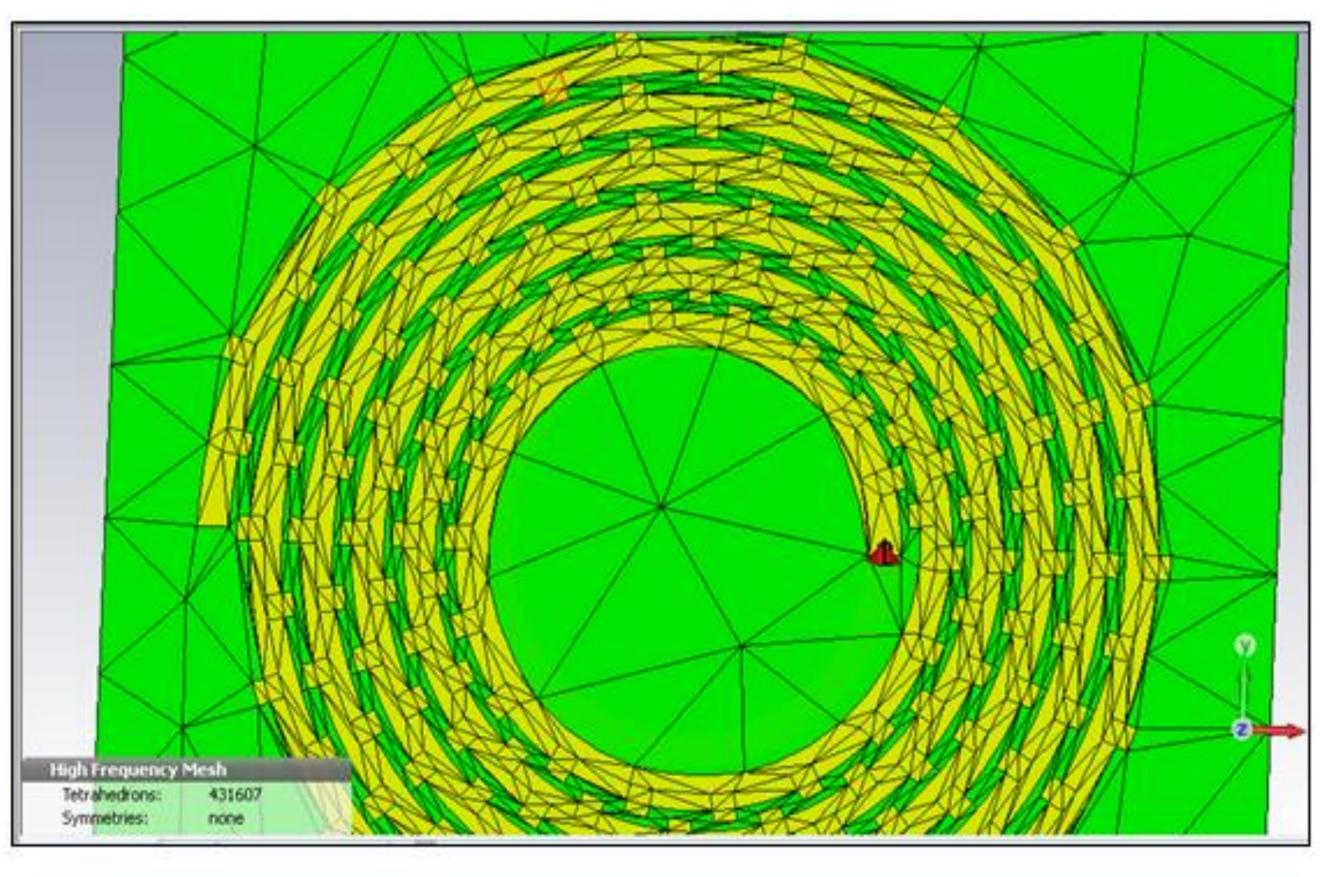
Figure 3 Spiral with inserted stubs, without Boolean add (Mesh View)
