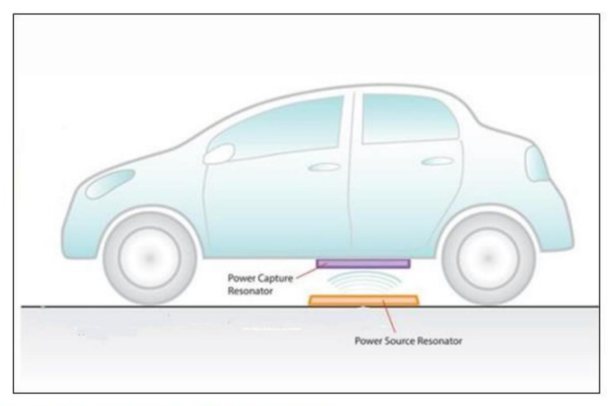
Figure 1 Electric Car with the Power capture and source resonators
