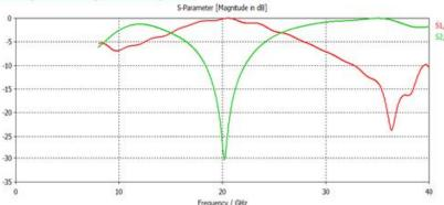
The simulation result shows a band stop filter with a resonant frequency fr = 20,22GHz . The relative bandwidth of the filter using -10dB as a reference is Brel [%] =  $\frac{3,87}{20,22}$  \* 100 = 19,14%
