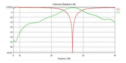
After the design and simulation of the above FSS array, the responses show a band pass filter with a resonant frequency , fr = 26,66GHz. The relative bandwith using -10dB as a reference is accordingly calculated as Brel [%] =  $\frac{1.94}{26,66} * 100 = 7,28\%$
